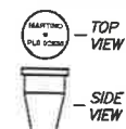
DETAIL OF TYPICAL CAP FOR 1/2"x18" REBAR SET BY PATRICK M. MARTINO, P.L.S.
